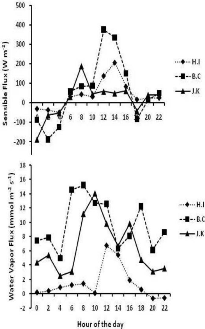
**Fig. 6.** Diurnal variation of sensible heat flux and water vapor flux in the three sites.
