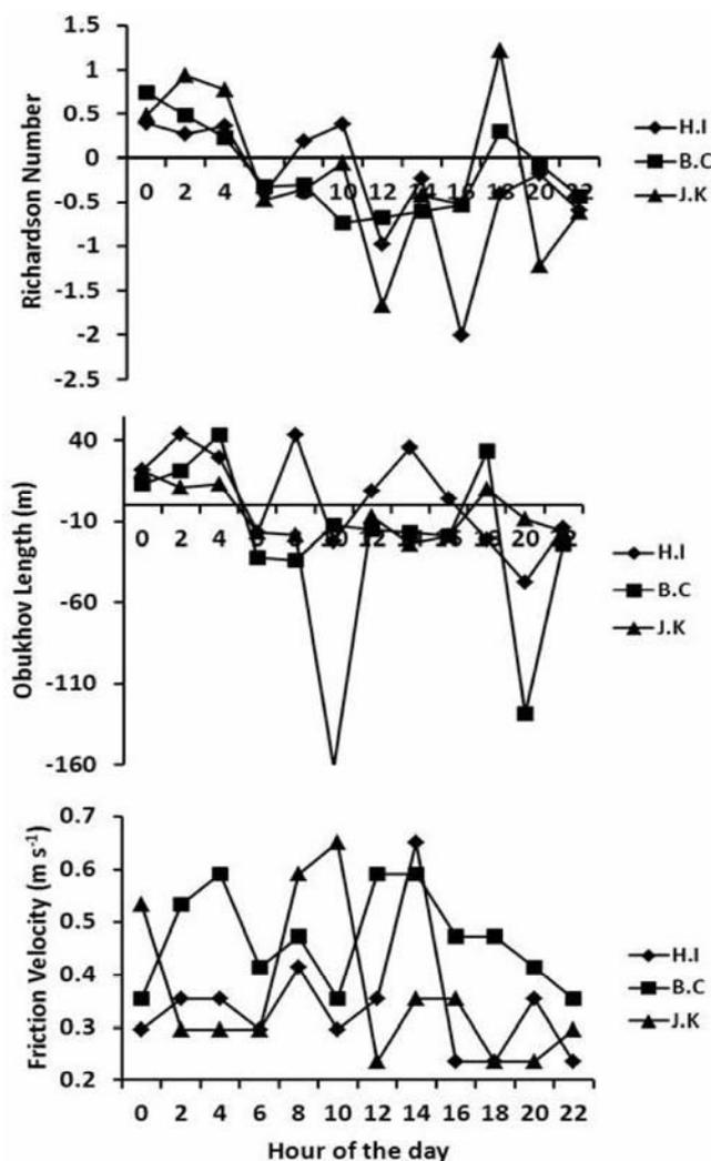
Fig. 2. Observed diurnal variation in Richardson number, Obukhov length and friction velocity (from top to bottom) in the three study sites.
